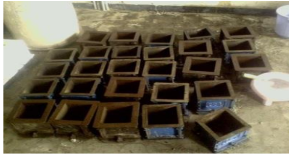
Figure 3: Arrangement of moulds
