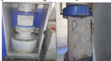
Figure 5: Testing cubes in compressive testing machine
